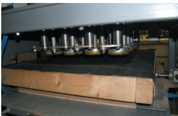
Figure 1 The current BDA Marathon Man test device
